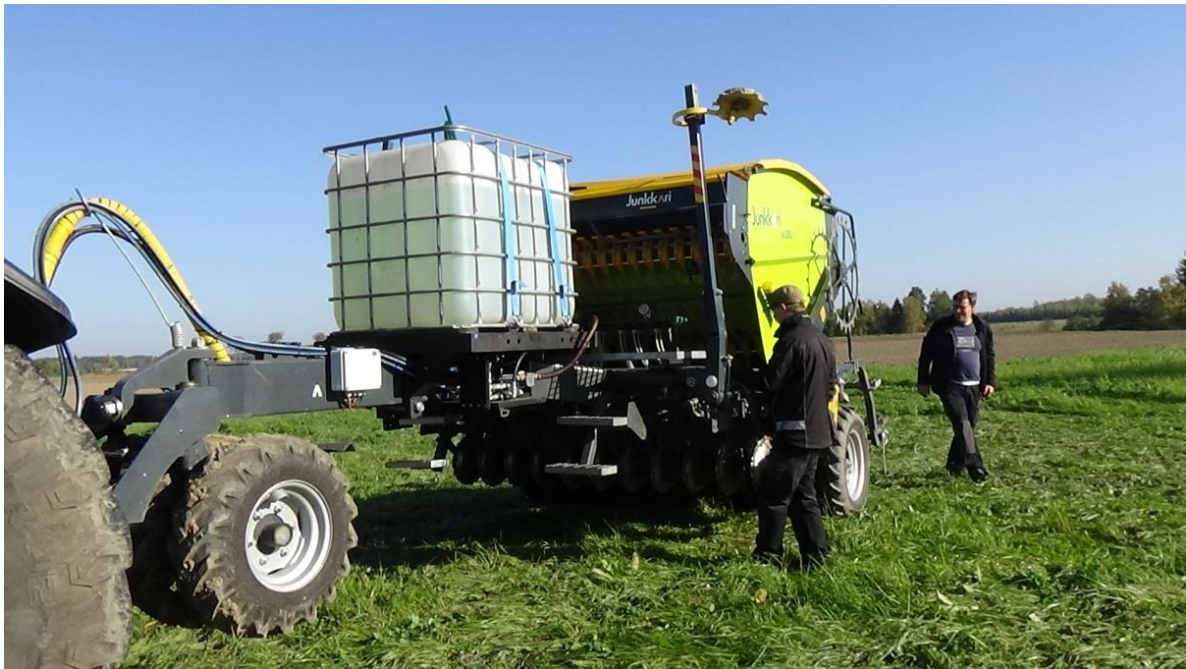
Fig. 1. AMS container on the CIRCWASTE combined seed driller system.
